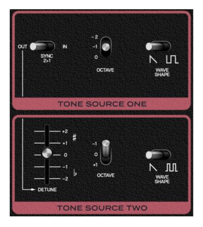
As monophonic analog synths go, MG-1 Plus is unique in that if features two standard mono analog oscillators (i.e., capable of sounding one note at a time), as well as a poly section that can sound up to 32 notes simultaneously. In this section, we'll discuss the mono oscillators. Note that the MG-1 front panel refers to oscillators as "tone sources;" perhaps Radio Shack felt this would be less intimidating for consumers than, "oscillator."
