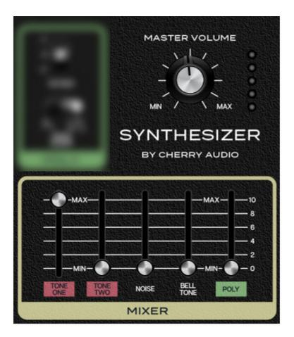
The Mixer section is where all MG-1 Plus signals are mixed together before going to the *Master Volume* control and onto the output.
