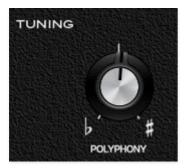
**Polyphony**- The second knob over at the top left of the panel acts as a master tuning control for the Poly section with a range of just over +/- 300 cents. This is also useful for subtle chorusing/detuning of the Poly section against the Tone Sources.
