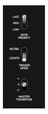
**Note Priority**- Since the Tone Generators are monophonic (i.e. they can only play one note at a time), this control determines which note will sound if more then one key is played simultaneously.
