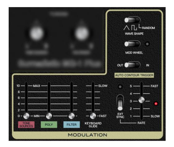
The MG-1 Plus includes a low-frequency oscillator (LFO) that generates subaudio range signals intended for modulation purposes.
