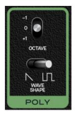
The original MG-1 included a rudimentary poly section that operated independently of the Tone Sources. The good news is that it allowed chords to be played on an otherwise mono (one-note-at-a-time) synth. The bad news is that it was extremely limited - its only control was a single level slider in the mixer section. It could only produce a square wave, its octave range was fixed, and its pitch could not be modulated. As you might guess, this made for a pretty blah poly synth experience.
