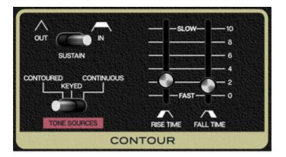
The envelope generator section is an envelope generator used to dynamically shape volume and and/or cutoff frequency. If you're not familiar with the operation of envelope generators, here's an overview:
